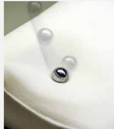
The material responds only slightly to energy applied to it, clearly demonstrating the pressure relieving effect of the visco-elastic foam.
